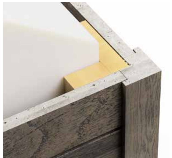
Fig. 8 - External corner detail
